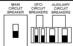
Figure 53. Main, AUX. and GFCI Circuit Breakers (OFF)
